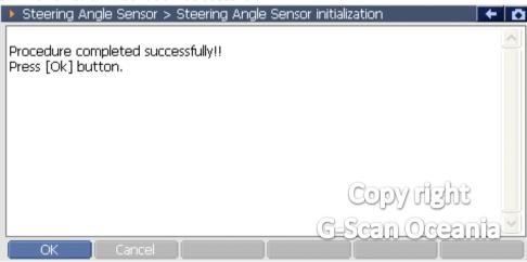
6. After initialization, Turn IGN OFF and wait 30 sec, turn IGN ON. The function will be completed.
